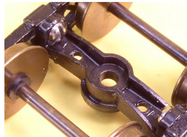
Equalized trucks allow the sideframes to pivot on the end of the bolster.
