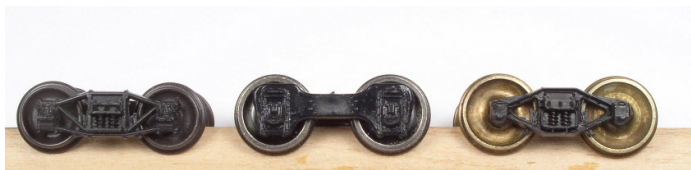
Rigid plastic HO trucks. Left to right: stock HO archbar truck, Fox style truck with Jay Bee 40" wheelsets, and with T-Section Bettendorf with NWSL 42" wheelsets.
