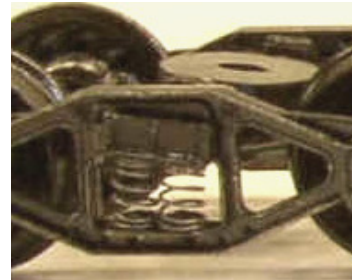
A sprung truck has working coil springs and the sideframes move independently of the bolster.
